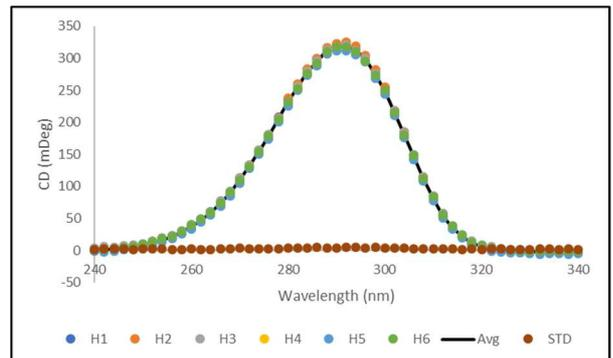
**Fig. 4.** Raw CD spectra of CSA from the final row of wells of an unskilled technician. The CD spectra of 200  $\mu$ l (+) CSA (Sigma) at 1 mg/ml in wells #A1-H12 of a solid silica bottom 96 well plate with black sidewalls (Porvair) from 240 - 340 nm were taken. Raw data were collected with no efforts to minimize the noise or evaporation at a room temperature of 25°C. Wells H1-H6 are shown in addition to the mean and standard deviation of those six.
