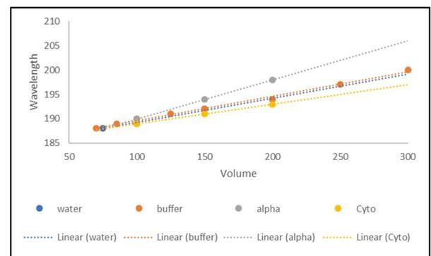
**Fig. 6. Cut Off Wavelength as a Function of Volume.** Replots of the cut off wavelength as a function of volume for H<sub>2</sub>O, K<sub>2</sub>PO<sub>4</sub> (10 mM, pH 7.4 Sigma), α-lactoglobulin (40 µg/ml Sigma) and Cytochrome C (40 µg/ml Sigma). Each point data point represents the STD of  $n \geq 12$  individual spectra.
