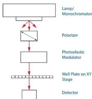
The EKKO™ CD Microplate Reader is a vertical CD spectrometer that turns the measuring light beam from the horizontal direction
