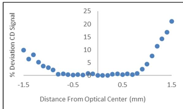
**Fig. 3.** % signal deviation as a function of distance from the optical center of the well. 200  $\mu$ l of CSA (Sigma) at 0.2 mg/ml was in well #F10 of a solid fused silica 96 well plate (Hellma). The CD signal was collected for 30 displacements of the beam path along the X-axis at 290 nm. Each position was 0.1 mm incrementally further away from the optical center of the well. Data is plotted as the % deviation from the mean.
