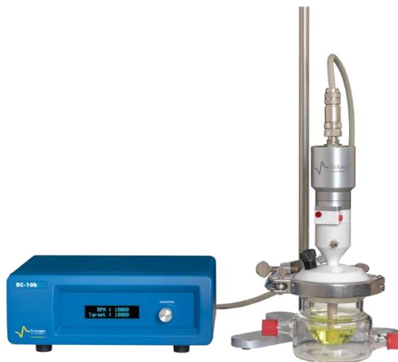
Figure 1: The BluRev RDE with EL-ELECTRO-1 and FeI/FeIII solution.
