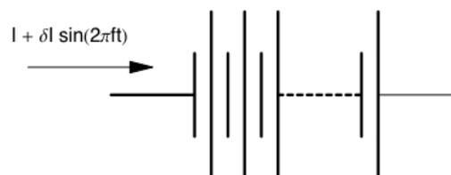
Figure 2 – Galvanostatic impedance measurement on a cell stack
