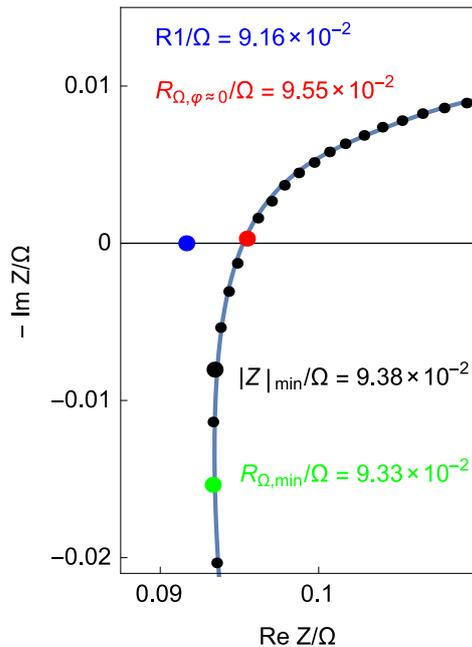
**Fig. 5: HF inset of the impedance graph of Fig. 2. Line: fitting result. Comparison of the various internal resistances obtained by single point measurement methods and by fit.**
