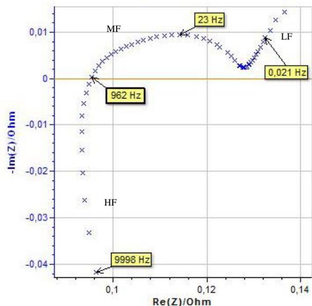
**Fig. 2:** Example of an impedance diagram of Li-ion battery. HF High Frequencies, MF Medium Frequencies, LF Low Frequencies.
