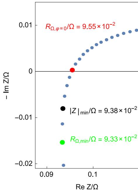
**Fig. 3:** Inset of the HF part of the impedance graph shown in Fig. 2. Comparison of the internal resistance measurement obtained using the impedance real part at minimal phase absolute value or zero phase (red dot), the minimal impedance module (black dot) or the minimal impedance real part (green dot).
