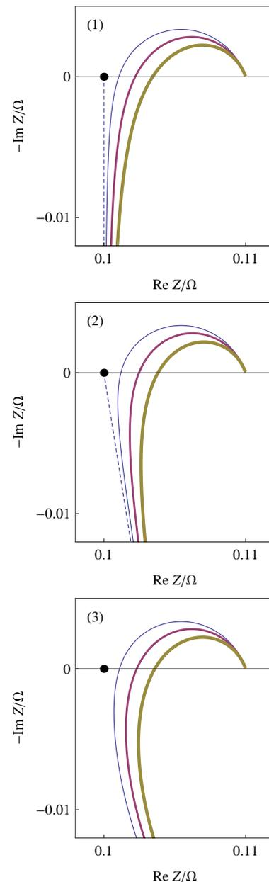
**Fig. 4: Change of impedance graphs of circuits  $R1+L2+R3/Q3$  (1),  $R1+La1+Q3/R3$  (2) et  $R1+L2/R2+Q3/R3$  (3) for various  $L1$  values. The thickness of the lines increases with  $L1$  and  $La1$  values. The black dot corresponds to  $R1$ .**
