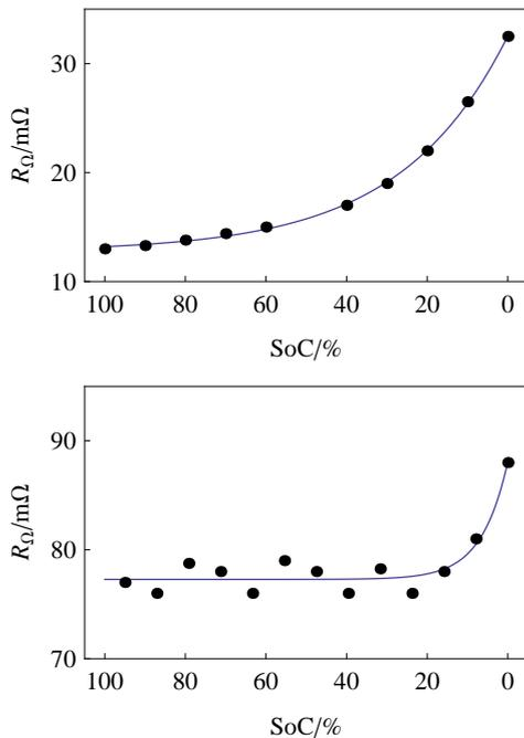
**Fig. 1:** Top: Change in internal resistance of a 6 V, 2.6 Ah lead-acid battery with SoC. Impedance measured at OCV. Figures taken from [6]. Bottom: internal resistance change vs. State of Charge (SoC) for a Mazda Ni-Cd type NCR6, 0.65 Ah battery through a 30 Ω constant load. Figure taken from [7].
