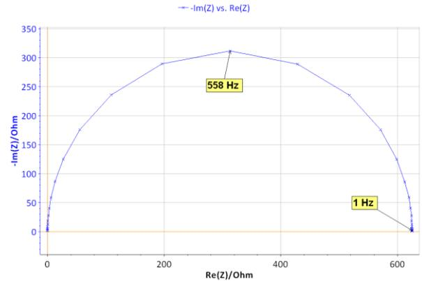
**Figure 8: Nyquist diagram of the impedance of the BP dummy cell measured at the rest potential (x),  $\delta E=10$  mV,  $f \in [500$  kHz, 200 mHz], and theoretical diagram of a R1/C1 circuit (line) with  $R1=624.4 \Omega$ ,  $C1=0.455 \cdot 10^{-6}$  F.**
