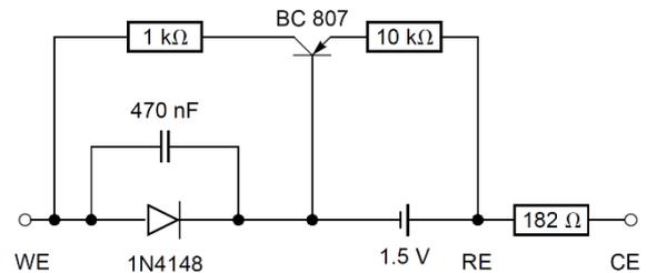
Figure 5: BP dummy cell.
