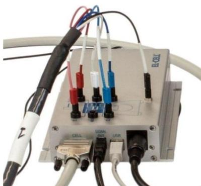
**Figure 4:** Cell cable connected to the data logger box.
