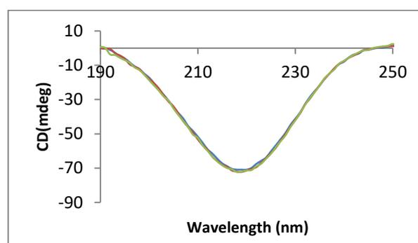
**Fig. 2. Raw CD spectra of systematically diluted PL with larger effective path lengths.** The CD spectrum of 200  $\mu$ l of PL (Sigma) at 0.1 mg/ml in well #F9 of a solid fused silica 96 well plate (Hellma) was recorded. The CD spectrum was then retaken after dilution with an additional 20  $\mu$ l of solvent added twice sequentially. Raw spectra were collected with no efforts to minimize the noise and were taken at a room temperature of 25°C.
