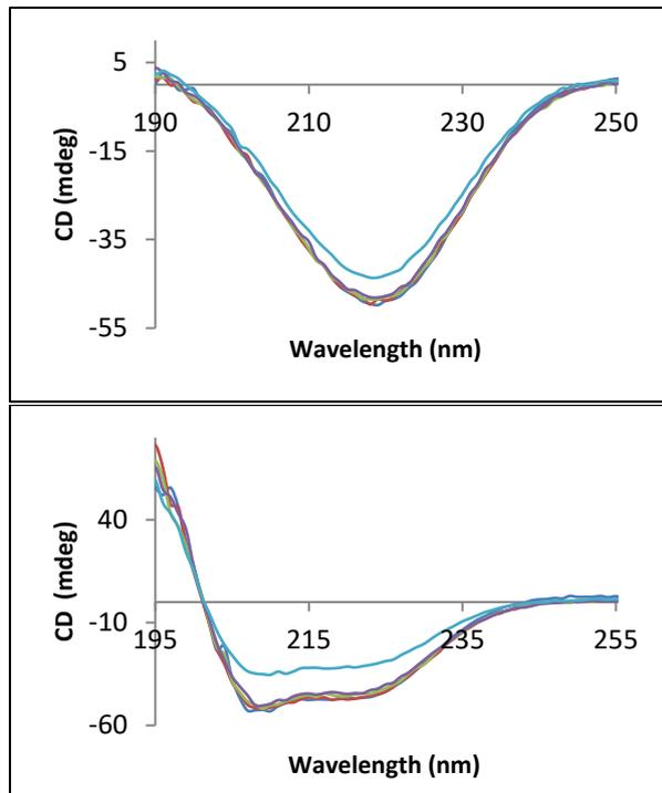
**Fig. 3. Raw CD spectra of PL (top) and BSA (bottom) with moderate effective pathlengths as a function of time.** 150  $\mu$ l of PL (Sigma) at 0.1 mg/ml in well #D9 and 140  $\mu$ l of BSA (Sigma) at 0.1 mg/ml in well #C10 of a solid fused silica 96 well plate (Hellma). Raw spectra were collected after 0, 2, 4, 6 and 23 hours of constant exposure to the environment of the sample chamber. No efforts to minimize evaporation at a room temperature of 25°C or noise were taken.
