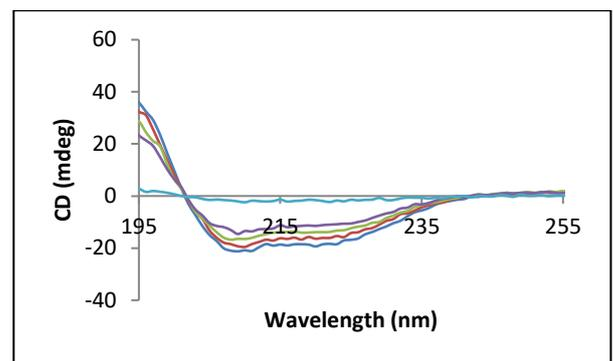
**Fig. 4. Raw CD spectra of BSA with shorter effective pathlengths as a function of time.** 70  $\mu$ l of BSA (Sigma) at 0.05 mg/ml in well #F8 of a solid fused silica 96 well plate (Hellma). Raw spectra were collected after 0, 2, 4, 6 and 23 hours of constant exposure to the environment of the sample chamber. No efforts to minimize evaporation or noise were taken. Room temperature was 25°C.
