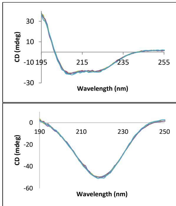
**Fig. 5. Raw CD spectra of BSA (top) and PL (bottom) with environmentally protected short effective pathlengths as a function of time.** 70  $\mu$ l of BSA (Sigma) at 0.05 mg/ml in well #F4 and 150  $\mu$ l of PL (Sigma) at 0.1mg/ml in well #D3 of a covered solid fused silica 96 well plate (Hellma). Raw spectra were collected after 0, 2, 4, 6 and 23 hours. No efforts to minimize noise were taken. The room temperature was 25°C.
