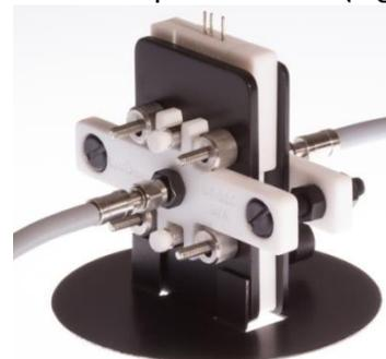
**Fig. 3:** Spectroelectrochemical cell with optical fibres.
