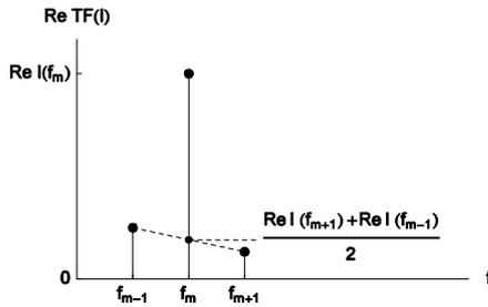
**Fig. 6: Principle of drift correction method for an imposed potential. (Real part of the Fourier spectrum).**
