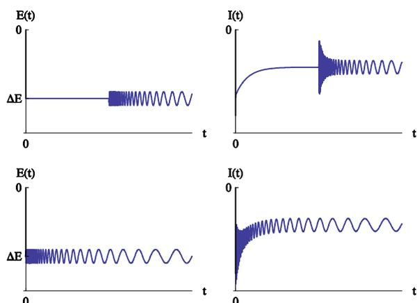
**Fig. 1: Example of a current response to an excitation by a sum of a potential step (amplitude:  $\Delta E$ ) and a series of sinusoids (amplitude:  $\delta E$ ). Left: sinusoids series starting when the steady state is reached. Right: sinusoid series starting at the beginning of the potential step.**
