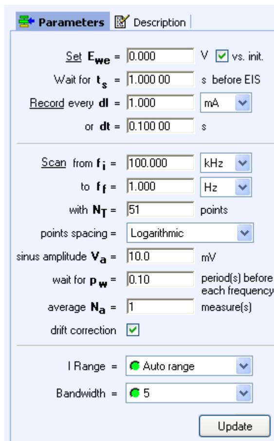
**Fig. 2: PEIS technique diagram in the EC-Lab® Express software with the drift correction box ticked.**
