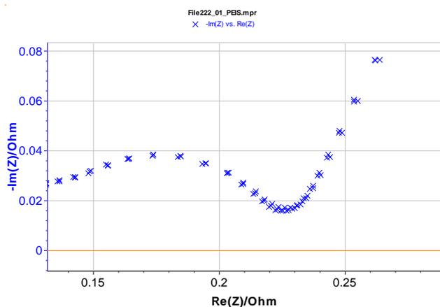
**Fig. 10: Lithium-ion battery impedance Nyquist graphs successively measured and low frequency enlargement; measurements done with drift correction. Same conditions as those of Fig. 9.**
