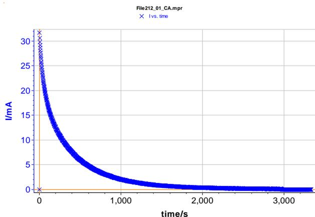
**Fig. 8: Lithium-ion battery current response to a potential step ( $E_{OC} = 3.09$  V).**
