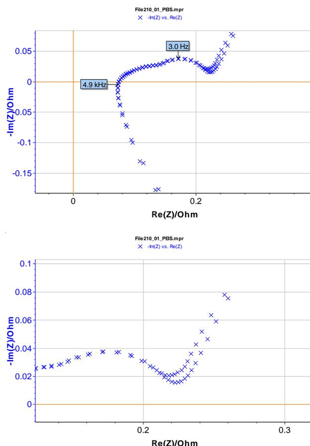
**Fig. 9: Lithium-ion battery impedance Nyquist graphs successively measured and low frequency enlargement. ( $f_{min} = 5$  mHz,  $f_{max} = 10$  kHz, 51 measurement points,  $\delta E = 3$  mV,  $E_{OCV} = 3.09$  V).**
