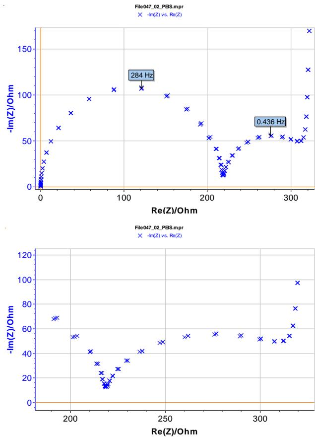
**Fig. 7: Three impedance Nyquist graphs with drift correction of Fig. 3 circuit measured successively from the potential step imposition.**
