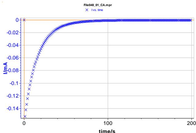
Fig. 4: Current response of the electrical circuit (Fig. 3) to a potential step.
