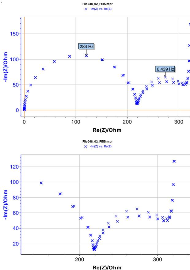
Fig. 5: Three impedance Nyquist graphs of the electrical circuit (Fig. 3) measured successively from the potential step application. Enlargement of the low frequencies area is also given. ( $f_{\min} = 20$  mHz,  $f_{\max} = 100$  kHz (51 measured points),  $\Delta E = 50$  mV,  $\Delta E = 10$  mV).
