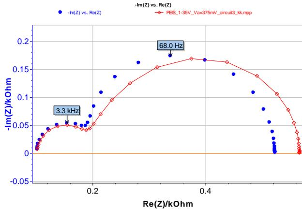
**Figure 3: Test circuit #3. Nyquist impedance diagram measured using PEIS technique.  $E_{WE} = -0.35$  V,  $V_a = 375$  mV,  $f_{min} = 0.2$  Hz,  $f_{max} = 50$  kHz (blue markers) and Nyquist impedance diagram obtained using KK transforms (red curve).**
