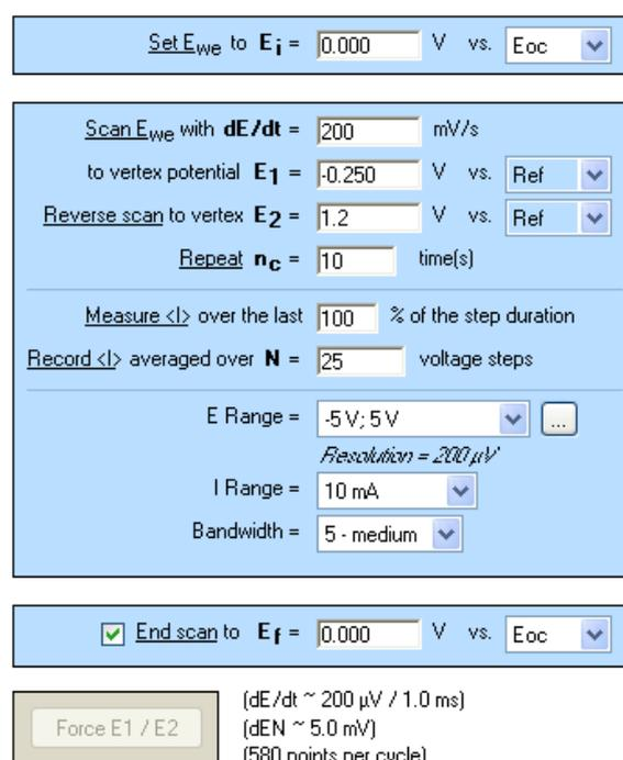
**Fig. 1: Cyclic Voltammetry "Parameters Settings" window.**
