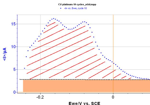
**Fig. 4:** Zoom of the curve presented in Fig. 3 for low potentials in oxidation. The red area corresponds to the desorption of hydrogen. The orange area corresponds to the capacitive current due to the double layer capacitance.
