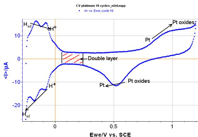
**Fig. 3:** 10<sup>th</sup> cycle isolated from the curve with oxido-reduction specificities for platinum.
