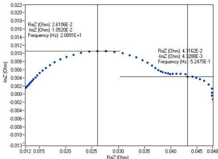
**Figure 7: The two capacitive arc at 20 and 0.5 Hz.**
