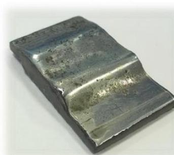
**Figure 6:** The steel weld measured by ic-SECM.
