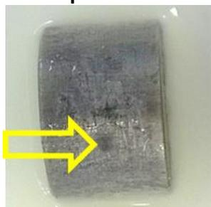
Figure 2: A convex portion of aluminium rod was measured by ic-SECM. The arrow indicates a blemish on the surface which affects the measurement.
