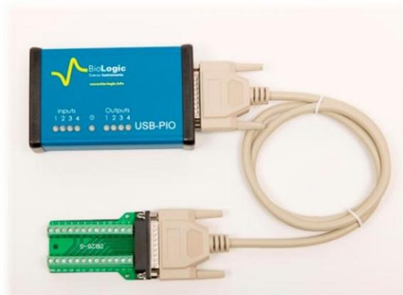
**Figure 2: The USB-PIO connected to the supplied break-out PCB. This image is representative only. The user should ensure their break-out PCB is correctly housed for their experimental setup.**
