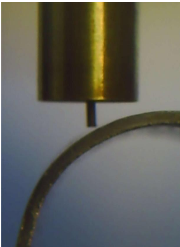
Figure 3 : Kelvin probe in close proximity ( \sim 220 \mu\text{m} ) to curved metal former. (Actual CTM and SKP experiment data taken with the probe at \sim 40 \mu\text{m} from the surface).
