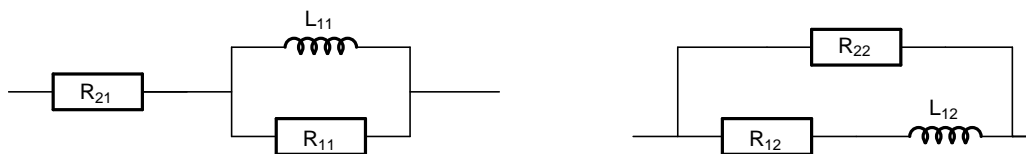
Figure 1.8: The (R+(R/L)) and ((R+L)/R) circuits are non-distinguishable.
