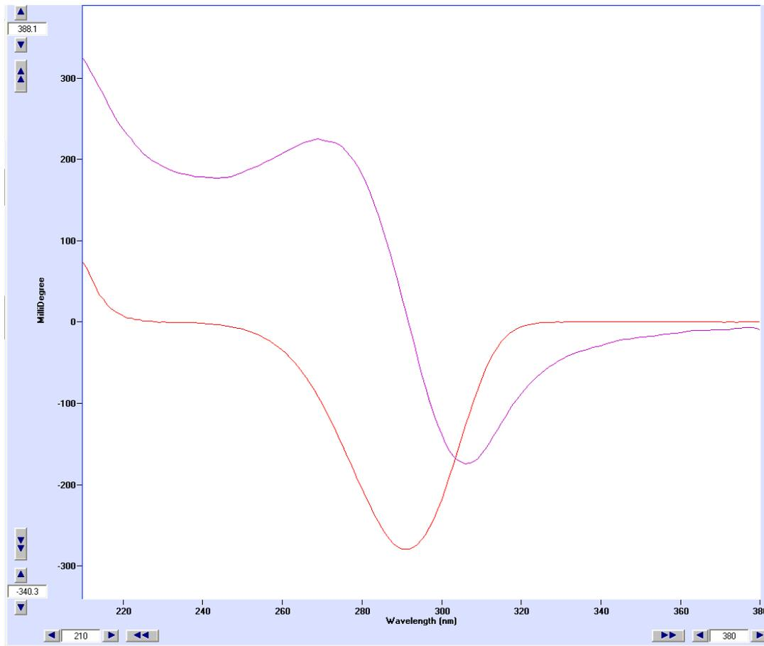
Figure 2: CSA (1S)-(-)-10-camphorsulphonic acid (0.9 mg/mL) in 1cm cuvette in water spectrum is displayed in both CD and ORD. Each plot has been performed using the MOS-450AF/CD from Bio-Logic SAS (France) at a fast sampling rate. Plot is only takes a few seconds.
