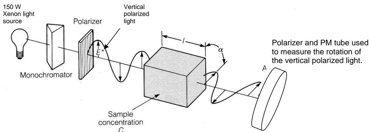
Figure 1: Simplified measurement set-up in ORD
