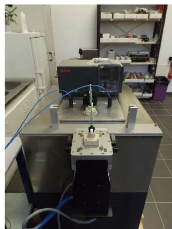
**Fig. 2 : stopped-flow attached to CS-90°C**
