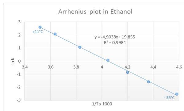
**Fig. 5 : Arrhenius plot in Ethanol**
