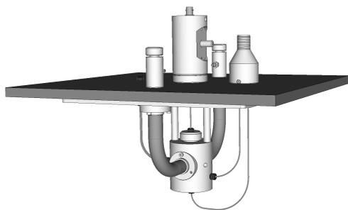
**Fig. 1 : cryo-mixing chamber
